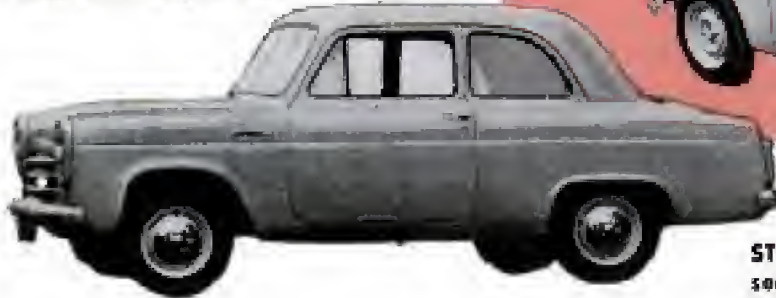
FORD introduces a new Anglia in England for '54, below. It has 4 cylinders, unitized body, gas tank in rear fender
